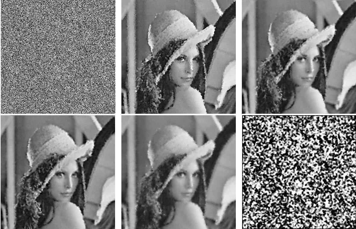
Fig. 4: Noisy image (95 % noise density) (top left), denoised by nearest neighbor interpolation (top middle), denoised by linear interpolation (top right), denoised by cubic interpolation (bottom left), denoised by linear finite element smoothing (bottom middle) and denoised by median filter (bottom right)
