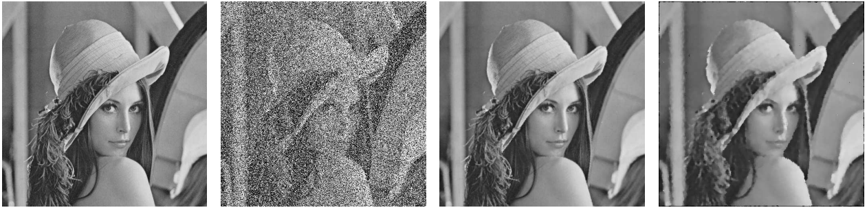
Fig. 3: Lena’s image (first), noisy image (noise density 50%) (second), denoised with linear interpolation (third) and denoised with median filter (last)
