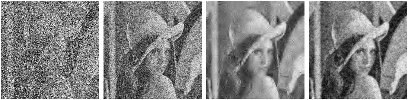
Fig. 6: Noisy image (first), image recovered by removing salt and pepper noise using finite element interpolation (second), image recovered by using wavelet smoothing in the second image (third) and denoised by linear finite element smoothing (last)
